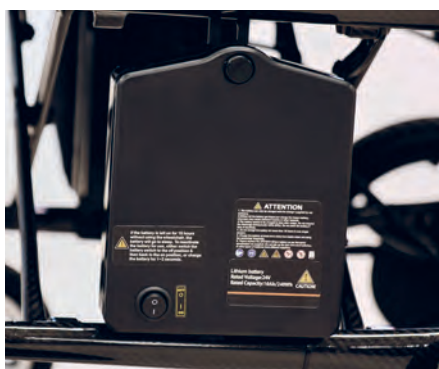
Lithium-ion airline friendly battery, 15km on one charge
